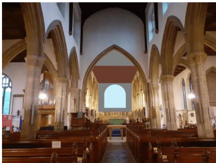
Figure 6. The chancel as would have been seen by Scott, with chancel arch blocked, lowered flat ceiling and smaller east window
