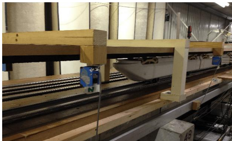
Figure 7 Upside down Eurostar model on the TRAIN Rig for underbody flow measurements
