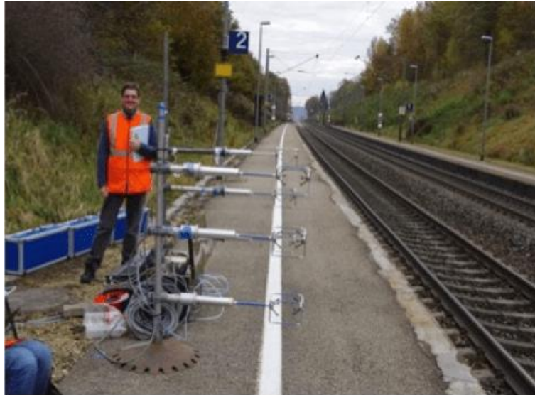
Figure 1 Slipstream measurements in Germany
