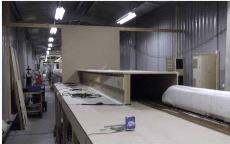
Figure 4 Tunnel entrance hood to eliminate sonic booms
